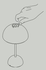
3. Remove the shade by unscrewing the dimmer knob and carefully lifting off the logo ring and upper shade. Check if the red and black wires are properly attached to the terminal block. This is done by gently pulling on each wire. If a wire comes loose, please reattach it by pushing down the button on top and fix the wire back in.
